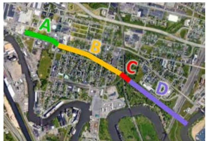
This image represents one potential arrangement for different uses and design needs for the trail and linear park based on geographic context. Section A has been flagged for a potential "rails-with-trails" configuration by the NFTA; Section B is in close proximity to homes and should be designed to consider appropriate privacy and screening; Section C will need to address how to traverse active rail lines; and Section D is most immersed in a park and natural setting and has direct access to the Buffalo River.
